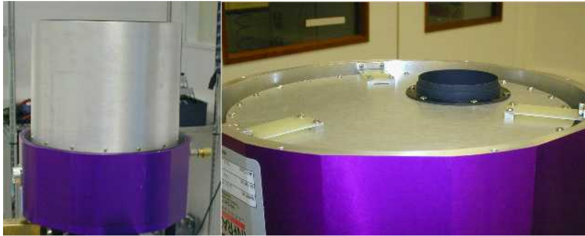
Figure 4: Assembled radiation shield surrounding detector mount & filter wheel (left) and a cover on the top radiation shield with supports (right)
