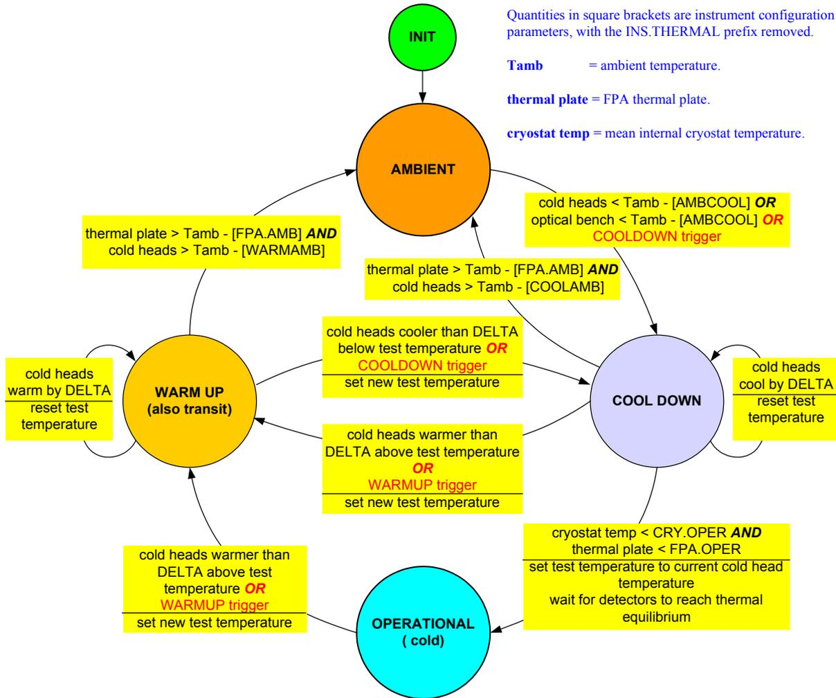
**Figure 3 VIRCAM Thermal Control States**
