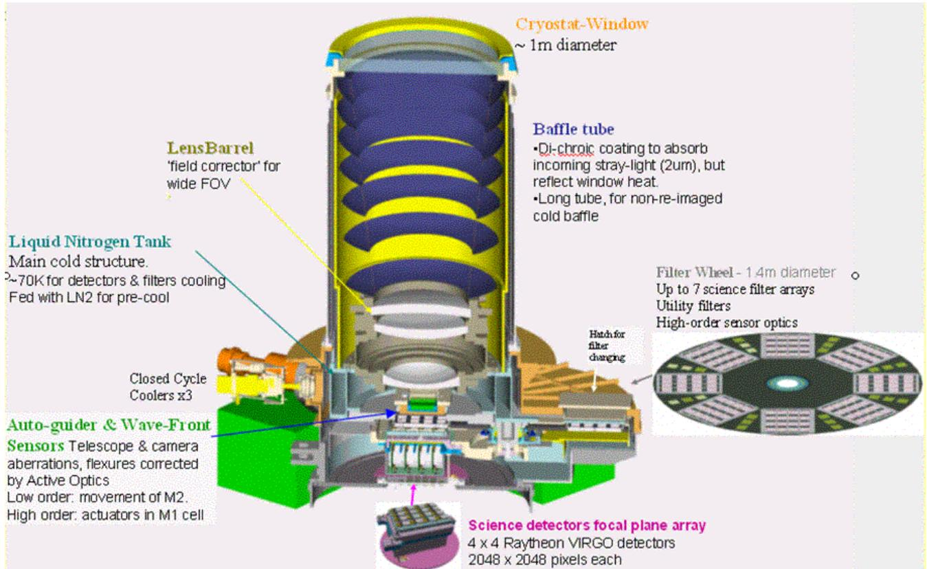
**Figure 1 Overall Layout of the VISTA IR Camera**
