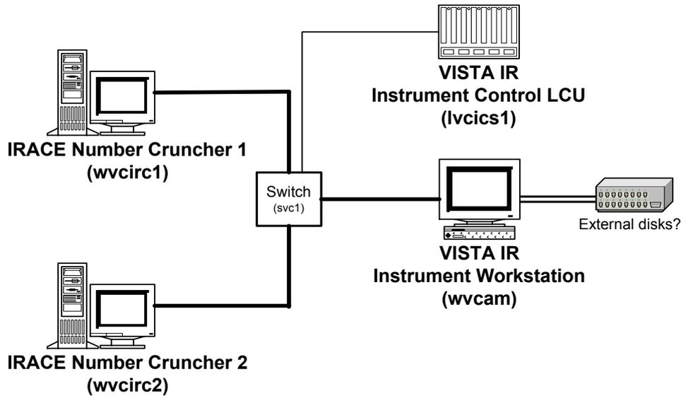
**Figure 22 Hardware required for stand-alone testing**
