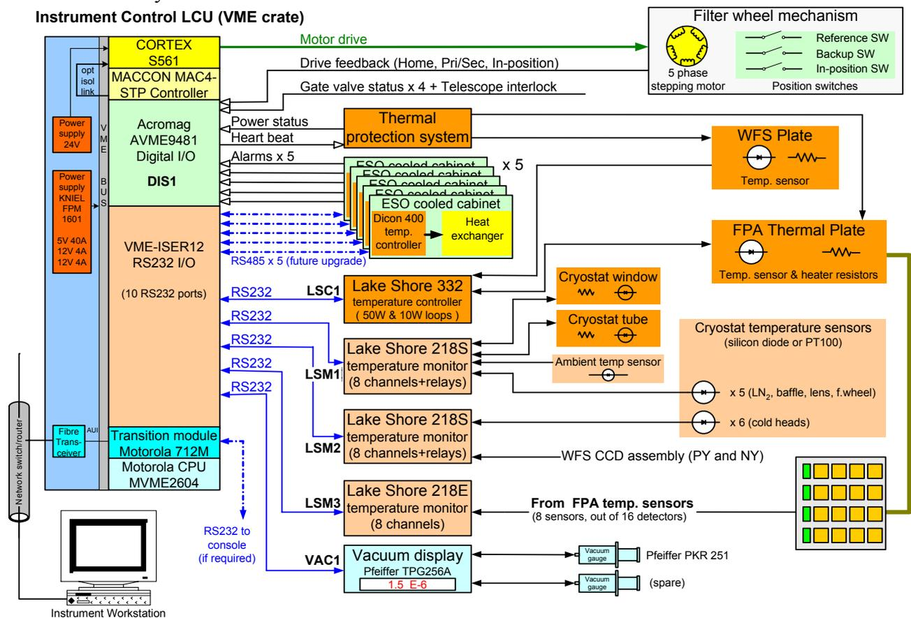
**Figure 2 Block Diagram of Instrument LCU Connections**
