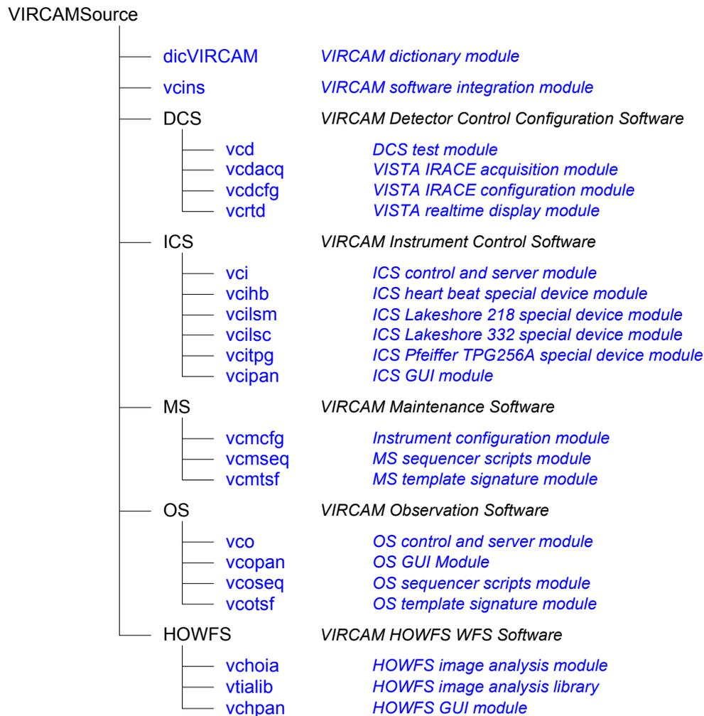
**Figure 18 VISTA IR Camera Software Modules and Source Layout**
