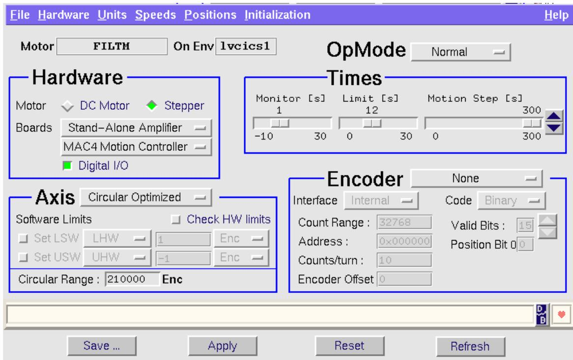
**Figure 43** motei Configuration Panel for VIRCAM Filter Wheel
