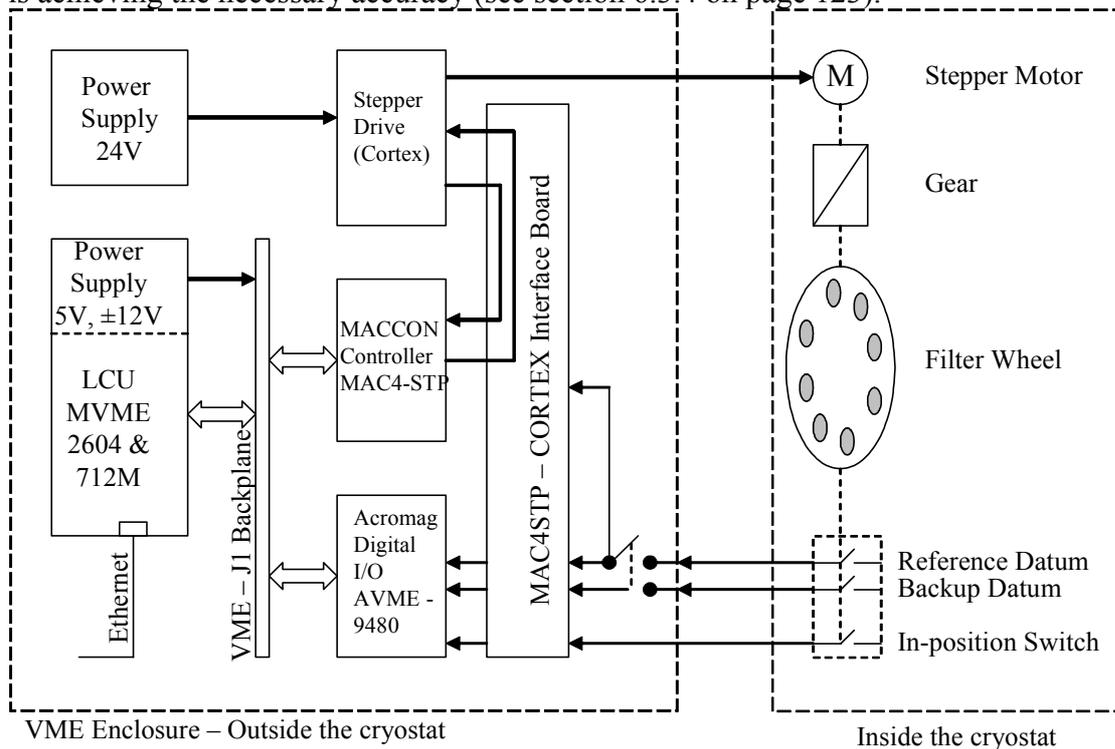
**Figure 5 Layout of the Filter Wheel Drive Electronics**
