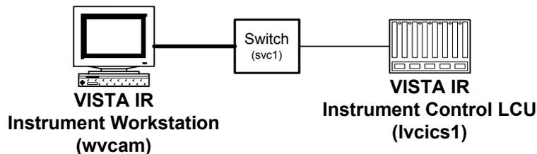
**Figure 20** Hardware required for LCU hardware simulation mode
