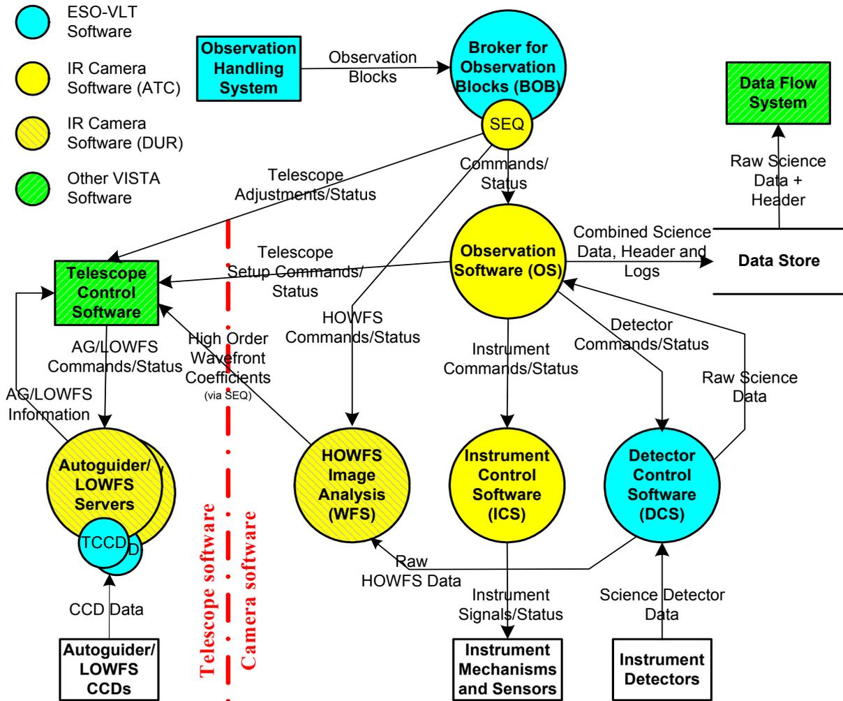
**Figure 17 VISTA IR Camera (VIRCAM) Software Architecture**
