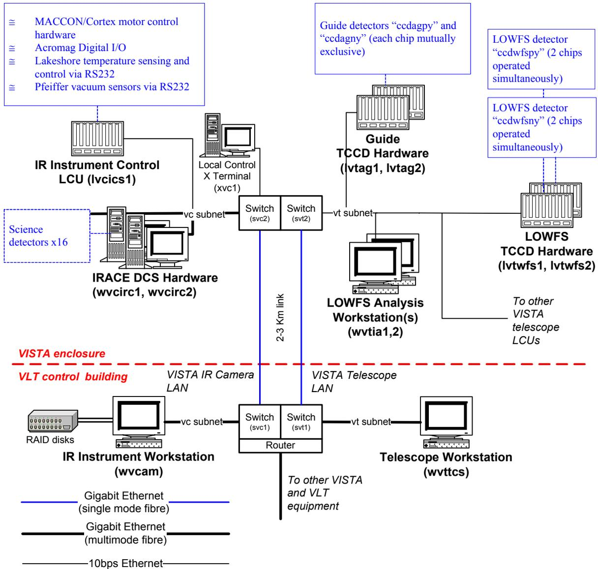
**Figure 11 Layout of the VISTA IR Camera LAN**
