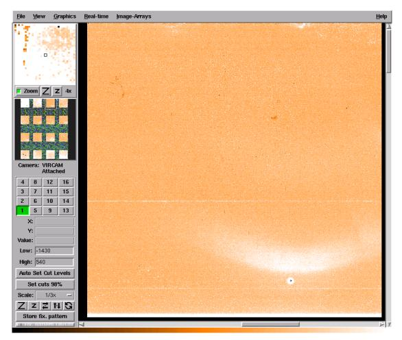
Residual image of Detector #42 showing the glow of the temperature diode. Peak count level is around 600 counts with a background of around 0.
