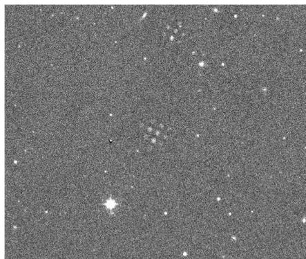
**Fig. 2.** Persistence effect (pattern of 9 decaying artefacts in the middle and upper middle) for a WFCAM frame following on after frames on M67.
