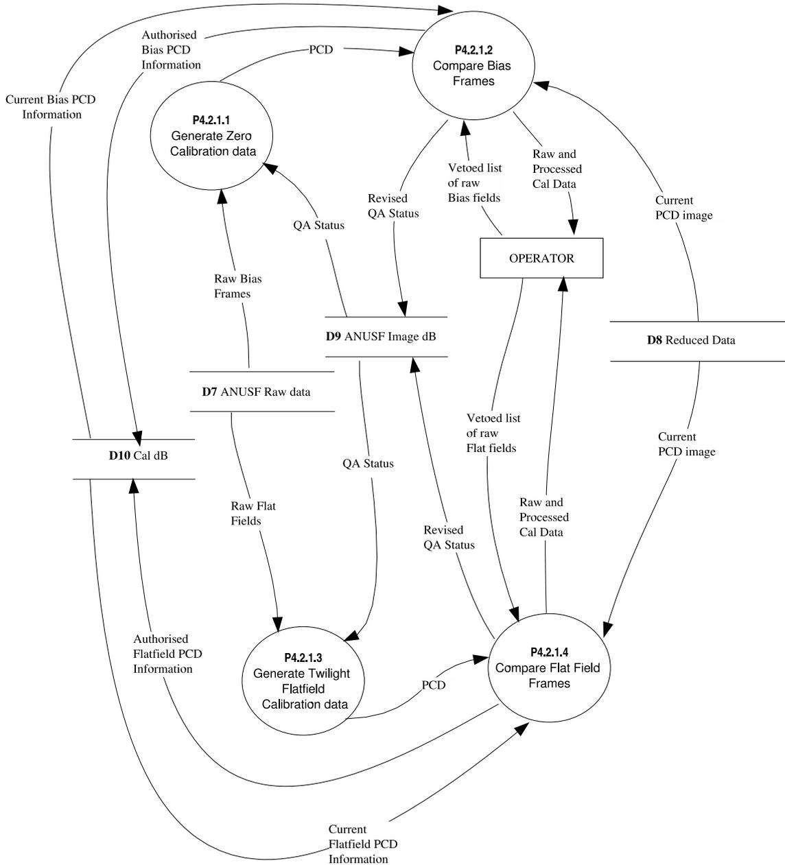
**Figure 8 Data flow diagram for P4.2.1 Calibration Quality Assurance**
