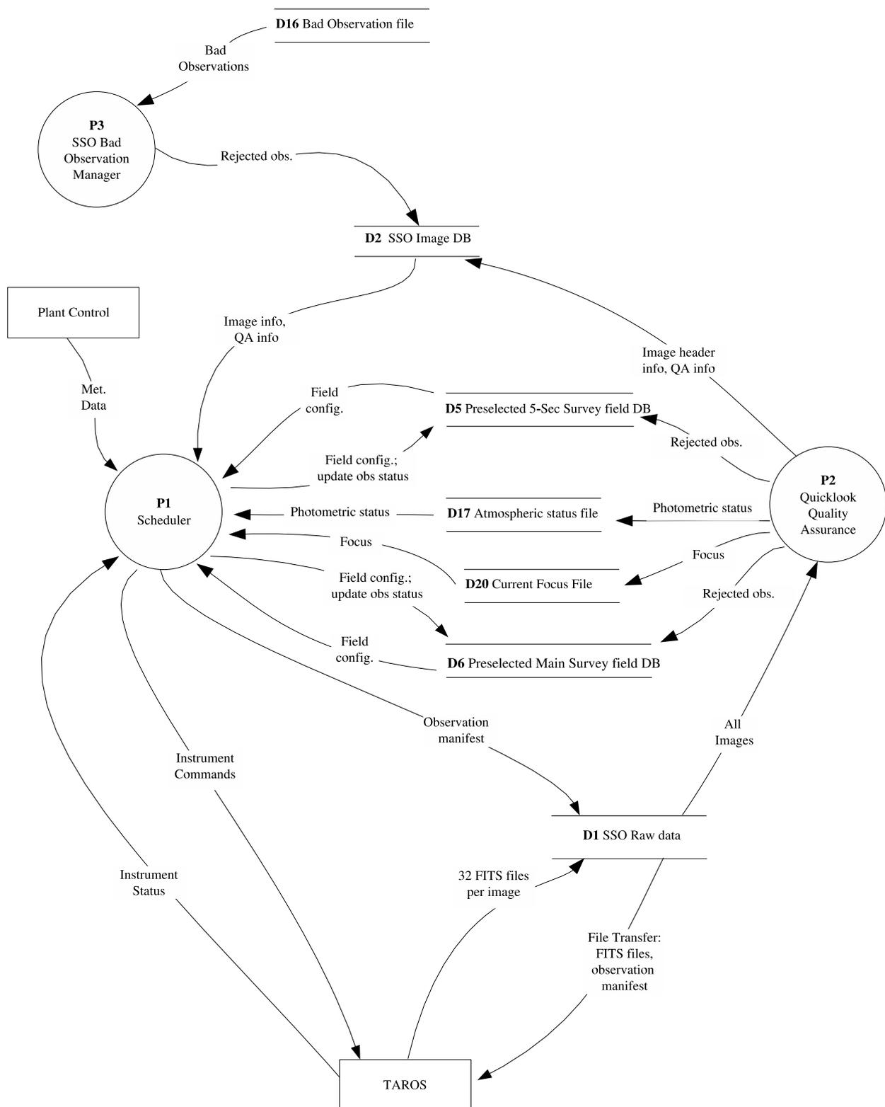
**Figure 3 System level data flow diagram for the Scheduler System**
