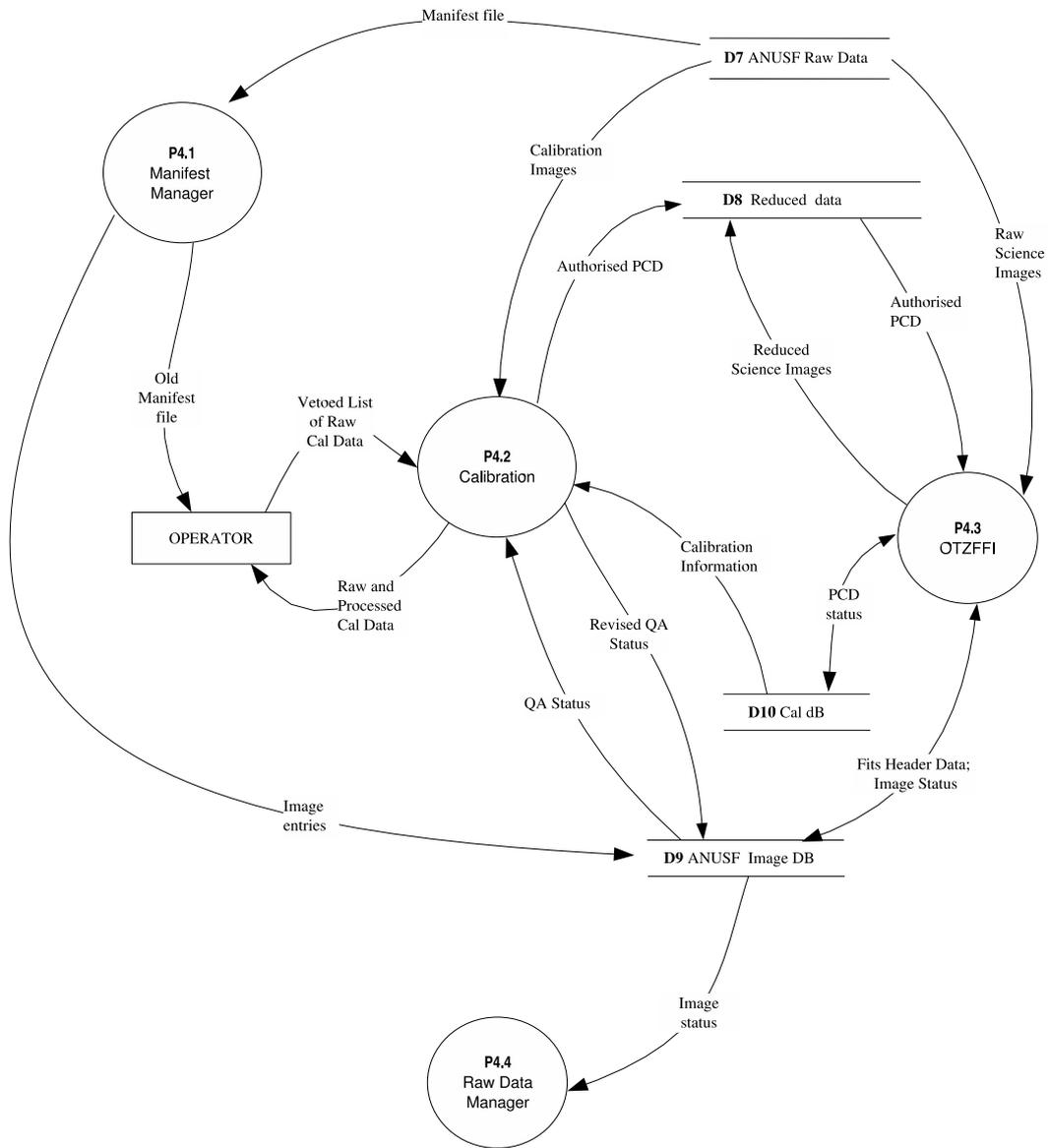
**Figure 6 Data flow diagram for P4 Data Reduction**
