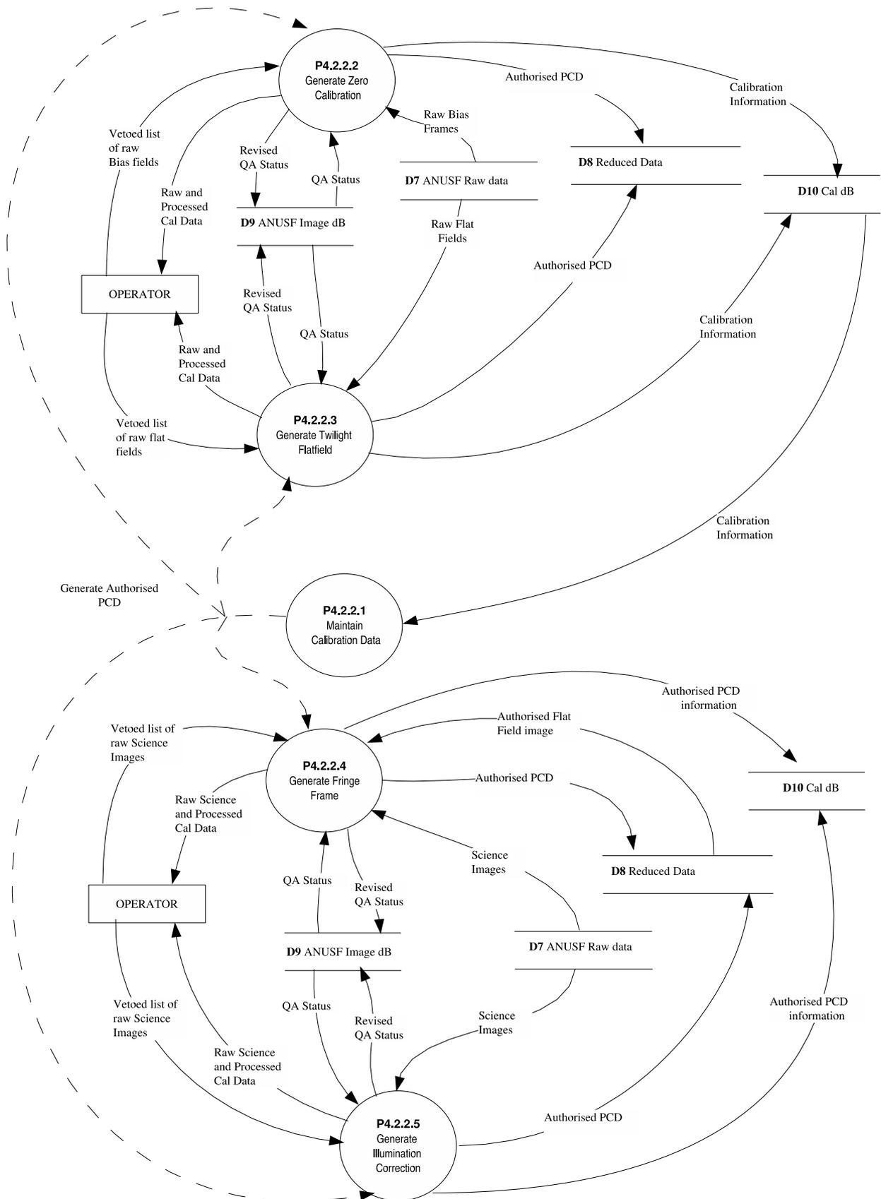
**Figure 9 Data flow diagram for P4.2.2 Generate Calibration**
