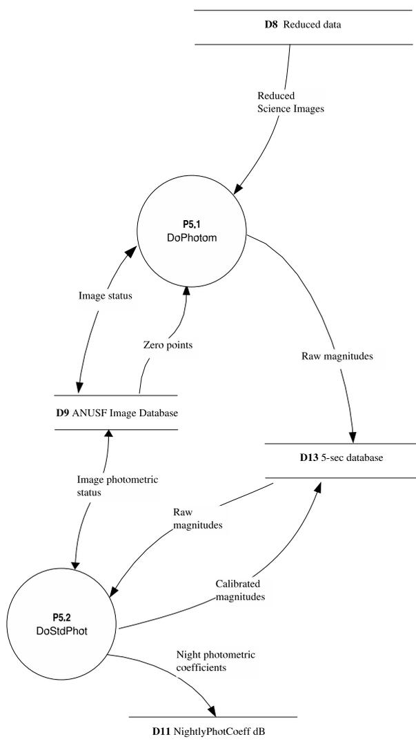
Figure 11 Data flow diagram for P5 5-Sec Survey Photometry
