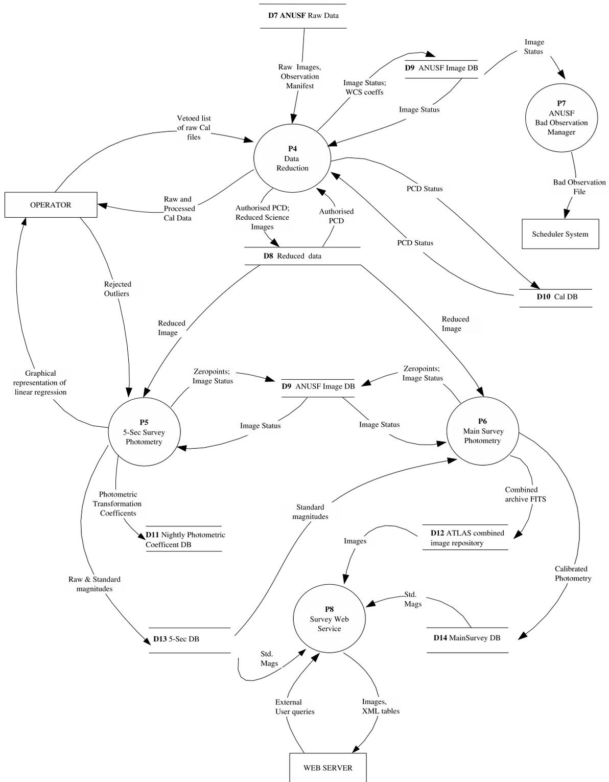
**Figure 5** System level data flow diagram for the Science Data Pipeline System
