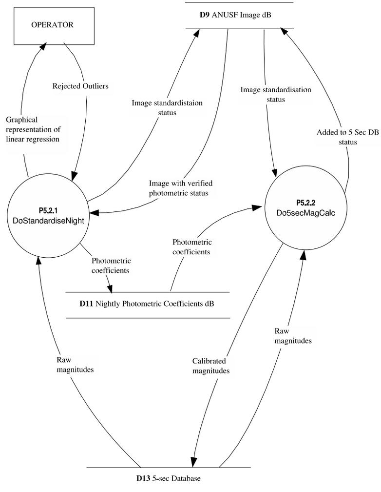
Figure 13 Data flow diagram for P5.2 DoStdPhot
