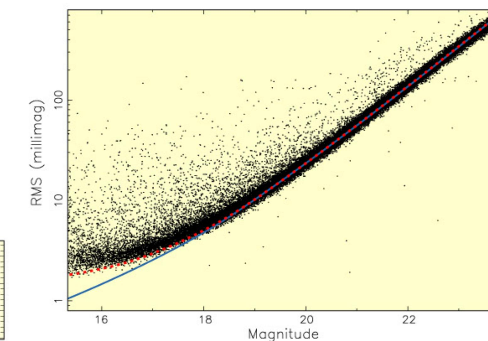
Figure 3: RMS scatter versus magnitude for all objects in the M50 field classified as stellar, obtained for the Feb 2005 CTIO data. The solid blue line shows the expected RMS, calculated as the quadrature sum of contributions from readout noise, sky noise in the photometric aperture and object photon noise. A dotted red line shows the same with a constant equal to 1.5 mmag added to account for residual systematic effects.
